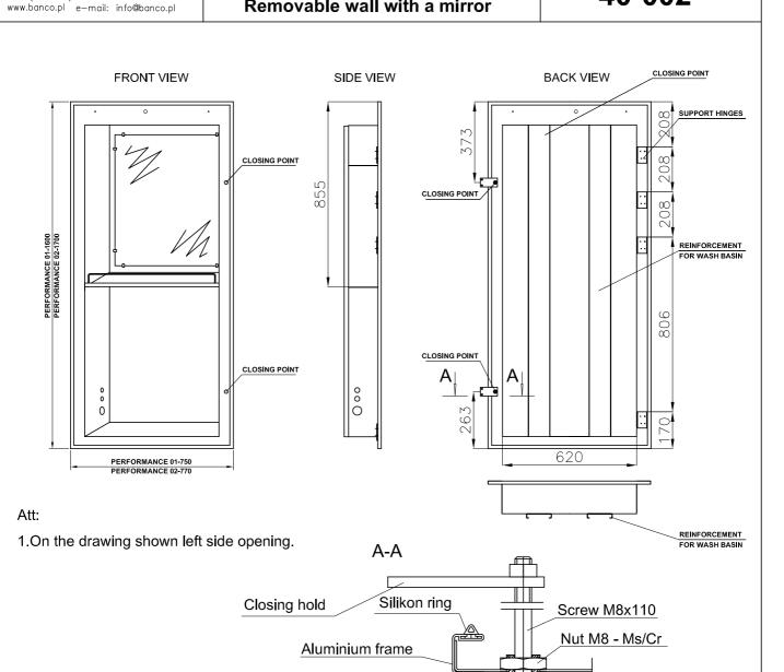
Metal swing wall is a part of the sanitary cabins equipment. It is mount to the wall of sanitary cabin by hinges and performs a function of locker and mirror.
