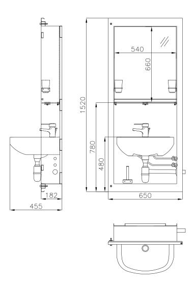
Metal swing wall is a part of the sanitary cabins equipment. It is mount to the sanitary cabin wall, attached by hinges and performs function of a locker and mirror.
